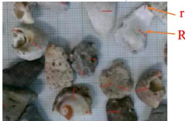
Figure 7: Measuring the radius of the sharpest corner of angular aggregate and the radius of circle inscribed in the aggregate using JMicrovision software.
