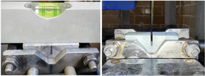
Figure 5. Notching the rock specimens
