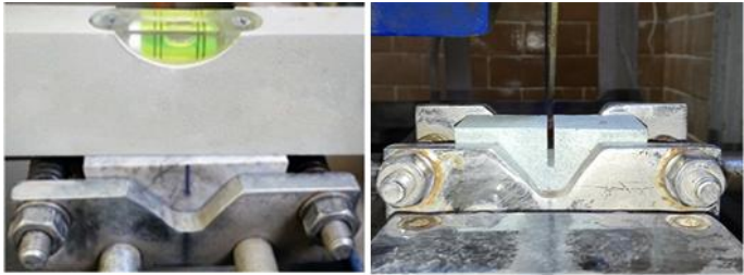
Figure 5. Notching the rock specimens
