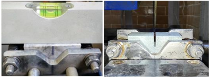
Figure 5. Notching the rock specimens
