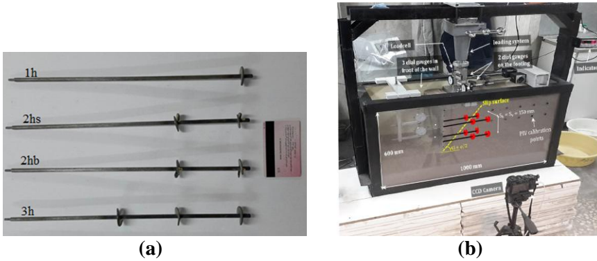
Fig. 4. (a) 4 Type of anchors used (b) Test box
