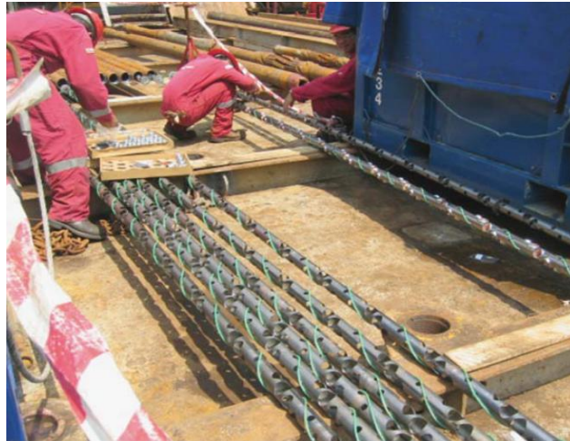
Figure 1. Loading shaped charges into perforating guns [6]
