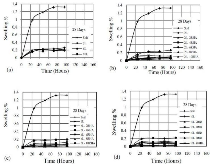
**Figure 9. Swelling potential of the stabilized gypseous clay with 28 days of curing time: (a) samples stabilized with lime; (b) samples stabilized with lime content of 2% and RHA; (c) samples stabilized with lime content of 6% and RHA; (d) samples stabilized with lime content of 10% and RHA**
