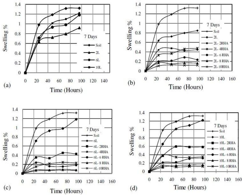
**Figure 8. Swelling potential of the stabilized gypseous clay with 7 days of curing time: (a) samples stabilized with lime; (b) samples stabilized with the lime content of 2% and RHA; (c) samples stabilized with the lime content of 6% and RHA; (d) samples stabilized with the lime content of 10% and RHA**
