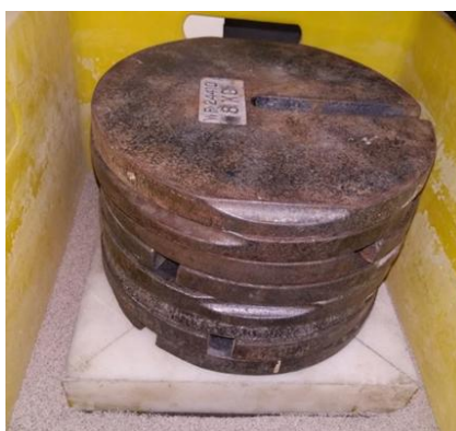
Figure 5. Method of roughening geotextiles
