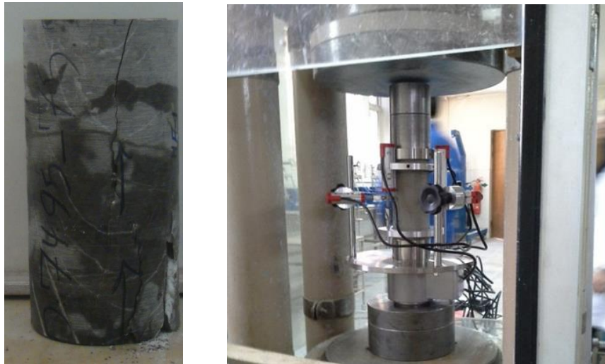
Fig.5. Examples of failure modes observed in limestone loaded in the Uniaxial Compression Test (Core specimens are ~82 mm in diameter)
