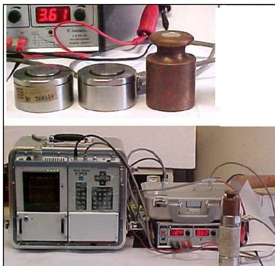
Fig. 4. Apparatuses of ultrasonic testing for determination of primary wave velocity ( V_p ), and shear wave velocity ( V_s )
