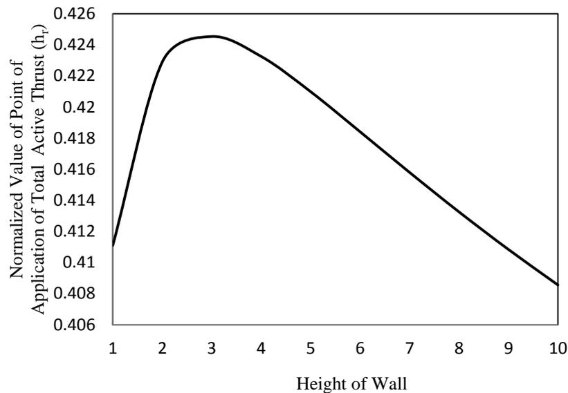
**Fig.7. Variation of height ratio of point of application of active thrust with height of the wall determined from present analysis for  $\varphi = 35^\circ$ ,  $H = 10 \text{ m}$ ,  $\gamma = 18 \frac{\text{kN}}{\text{m}^3}$**
