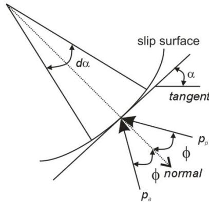
Fig.1. Pressure applied on failure surface for cohesionless soil in active and passive conditions
