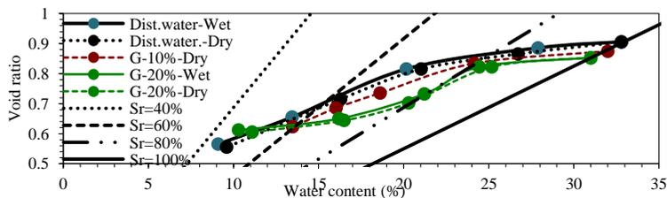
**Figure 2. Water content-void ratio paths for different quality of flooding fluids**
