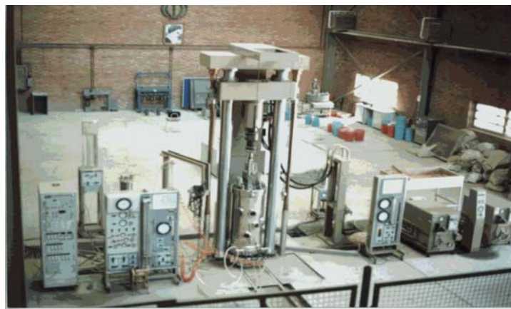
Fig 2. Large triaxial apparatus
