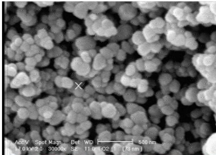
Fig. 3. SEM image of TiO<sub>2</sub> thin film (the average grain size is 73 nm)
