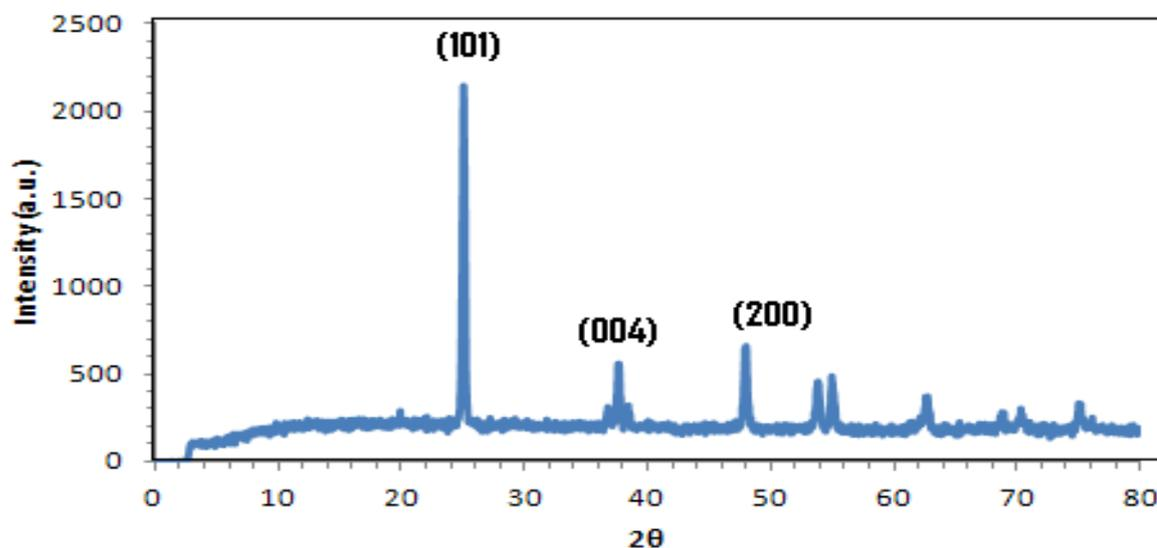
**Fig. 2. XRD pattern of TiO<sub>2</sub> thin film**
