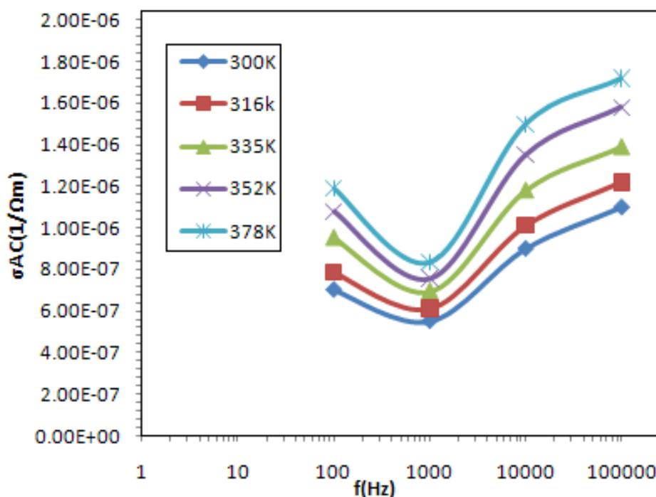
**Fig. 5. Dependence of AC conductivity on frequency at different constant temperatures**
