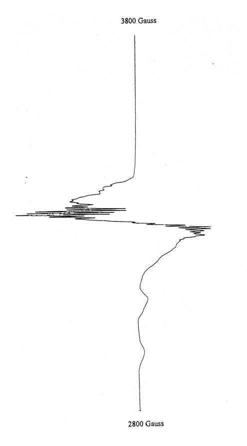
Figure 3: ESR spectra of complex [Cu<sub>2</sub>L<sub>1</sub>] at room temperature. The field set was 3300 gauss, and the scan range was 1000 gauss.
